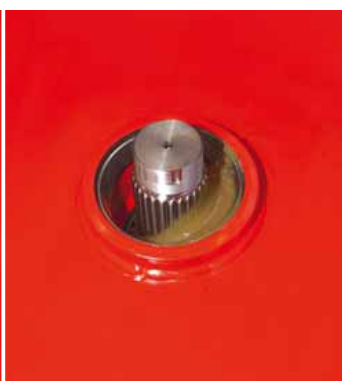
50 of 60 mm dikke assen en grote kegellagers
